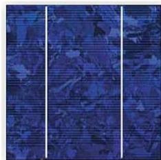
Fig. 1.11-Cella in silicio policristallino
