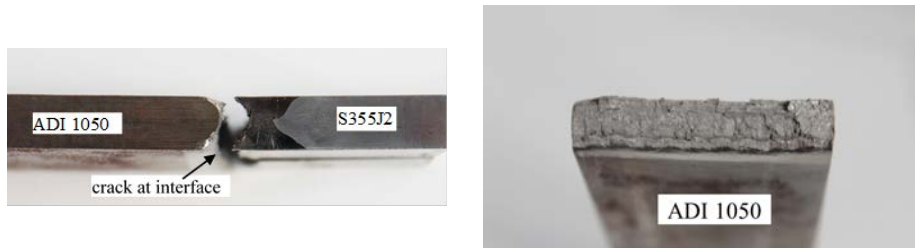
Figure 6.5: Fracture surfaces of full-penetration ground butt-joints : specimen B2-4,as welded, axial loading, R=0.05 , \Delta\sigma = 320MPa , N_f = 109630cycles
