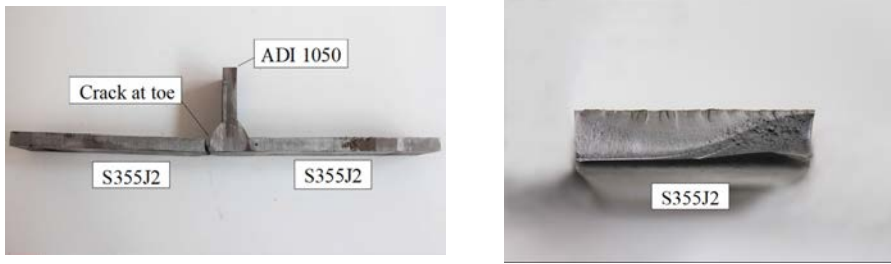
Figure 6.9: Fracture surfaces of T non-load-carrying fillet-welded joints: specimen D1-1, as welded, axial loading, R=0.05 , \Delta\sigma = 234\text{MPa} , N_f = 353034\text{cycles}
