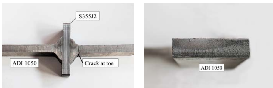
Figure 6.7: Fracture surfaces of cruciform load-carrying fillet-welded joints: specimen E3-1,as welded, axial loading \Delta\sigma = 208MPa , N_f = 118526cycles
