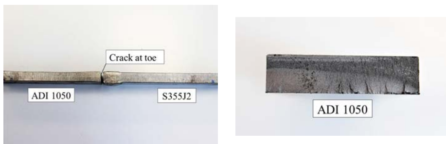
Figure 6.4: Fracture surfaces of full-penetration butt-joints : specimen B2-6, as welded, 4PB loading, R=0.05 , \Delta\sigma = 293.6MPa , N_f = 331582cycles
