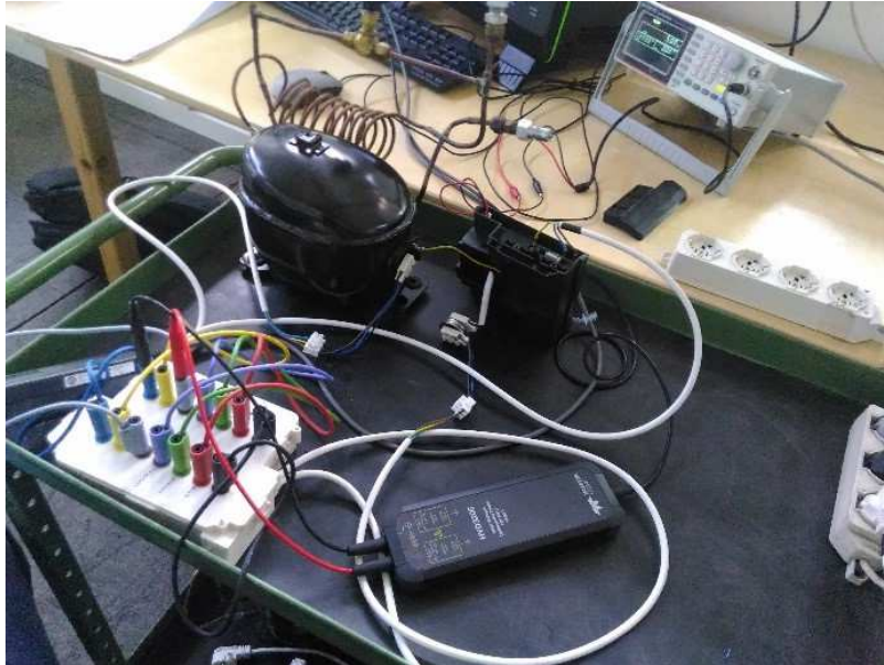
(a) Initial setup. The differential voltage and current probes connected to the Motor Drive Analyzer can be spotted (Sec.4.2.1).
