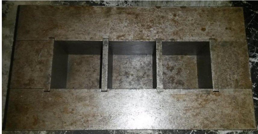
Figure 5.23: Mould used to cast the specimens for compression testing.
