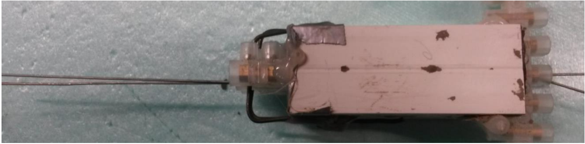
Figure 6.2: 60 mm pull-out specimen containing 2 twisted wires.
