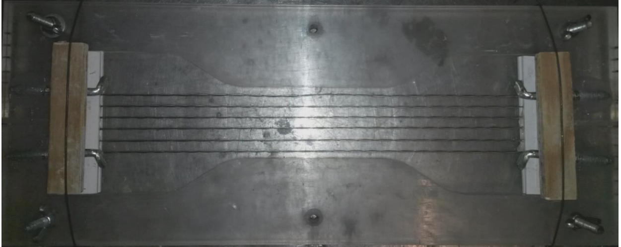
Figure 6.20: Twisted wires placed in the mold. The plastic plates were fixed using “L” screws, hot glue, small wood pieces and steel wire.
