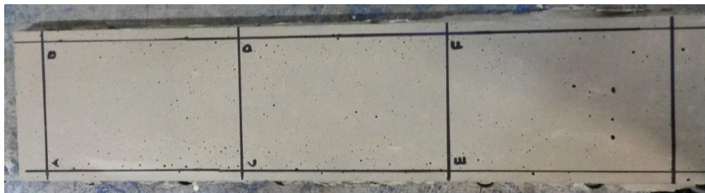
Figure 5.4: Position of the specimens in the plate before cutting.
