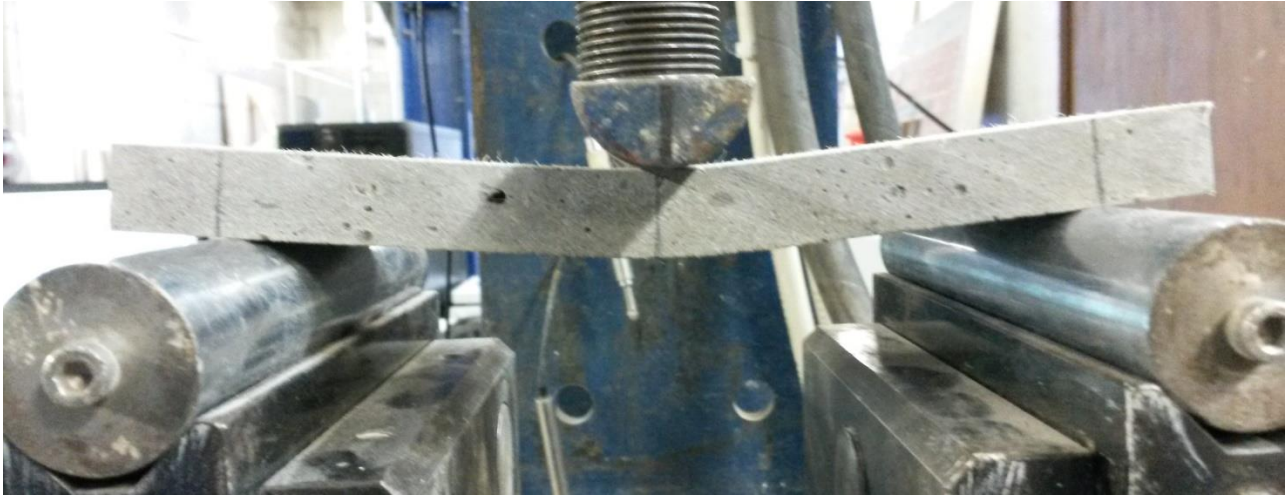
Figure 5.27: ECC specimen during flexural testing.
