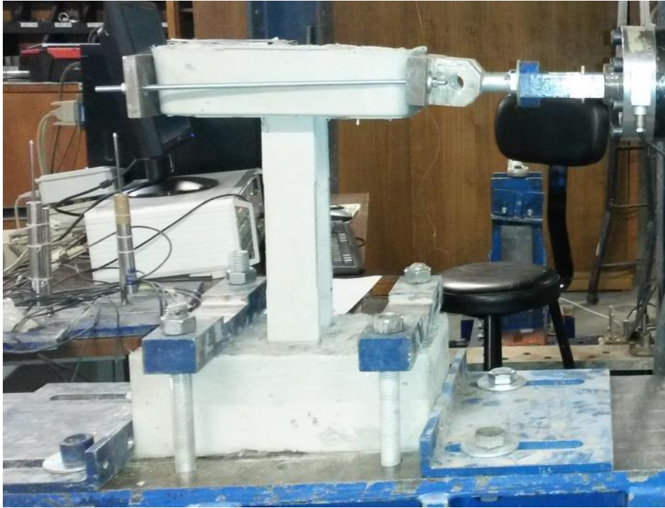
Figure 6.29: Column and actuator.
