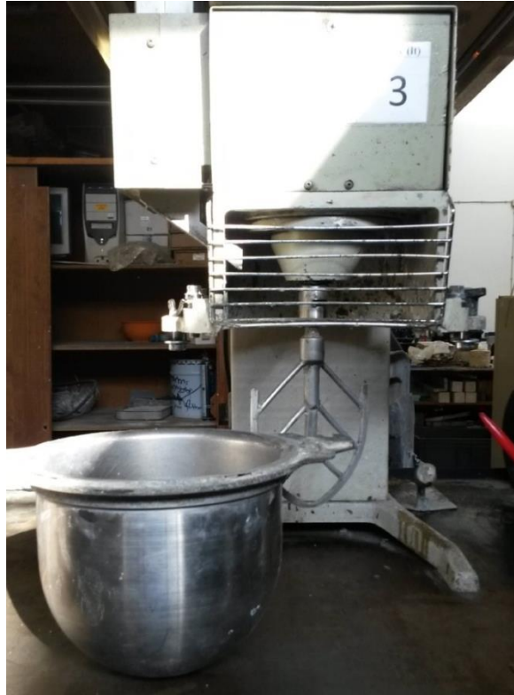
Figure 5.1: Automatic mixer, spoon and bowl used to mix the materials.
