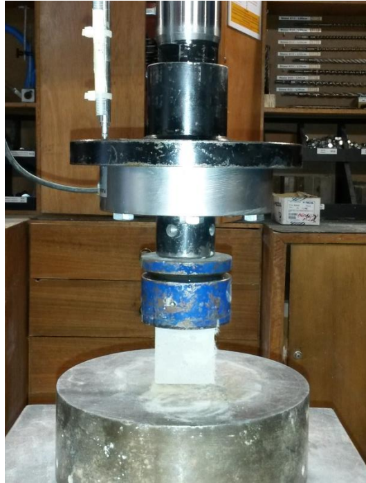
Figure 5.25: Test setup used for the compression tests. The cross-head displacement was measured using one LVDT.
