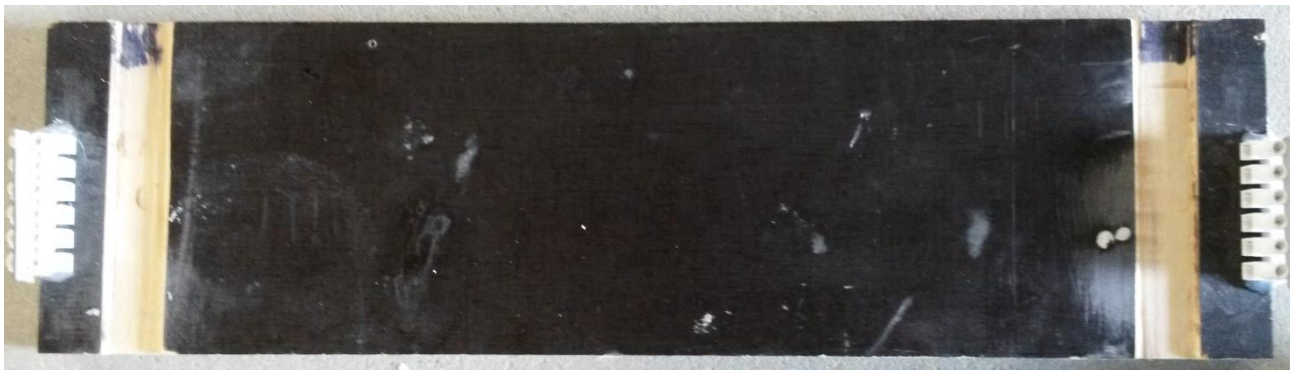
Figure 6.17: Wood plate with the connectors fixed at the edges using super glue and hot glue.
