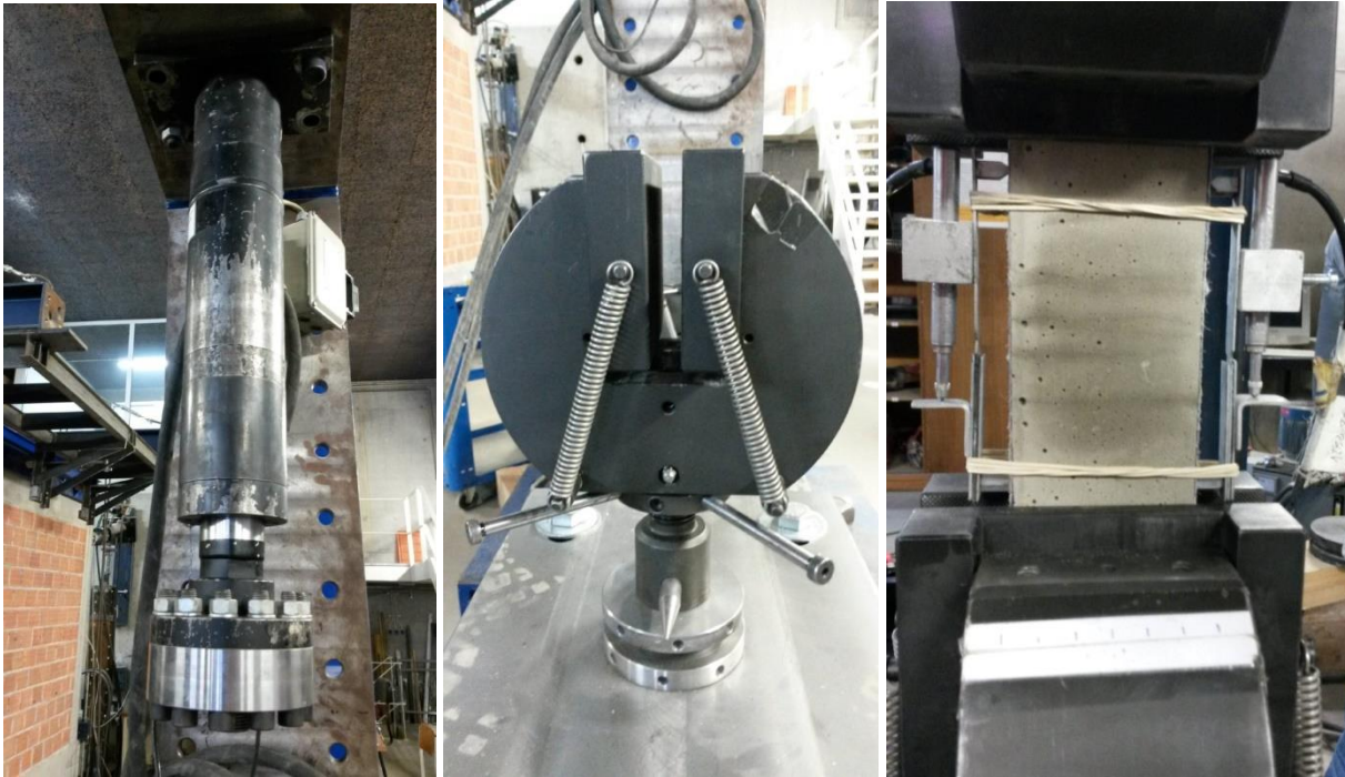
Figure 5.5: Actuator and load cell (a), clamping device (b) and clamped specimen during the test (c).
