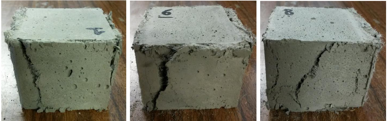
Figure 5.26: Three cubic specimens after compression test.
