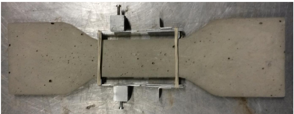
Figure 5.31: Dogbone-shaped specimen before testing and the 2 devices used to place the 2 LVDT.
