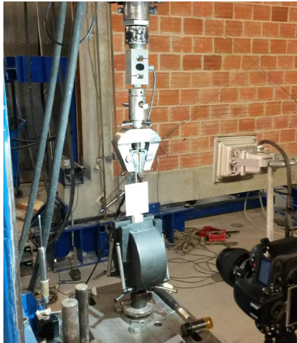
Figure 6.6: Setup used to capture high resolution images during pull-out testing.
