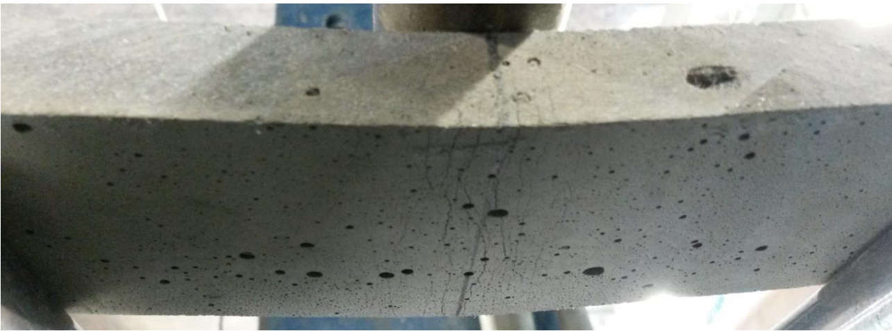
Figure 5.28: Formation of micro-cracks on the bottom of the specimen.
