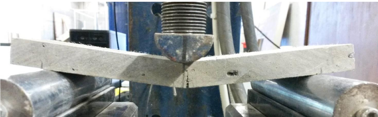
Figure 5.29: Formation of a large crack and failure of the specimen.
