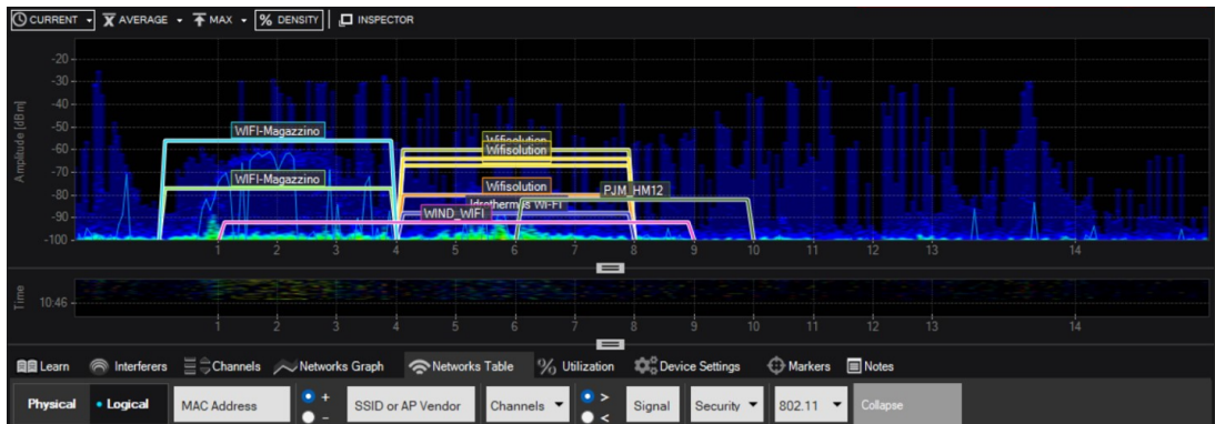
Figure 5.1: Example of wireless sampling performed with a laptop antenna, without the help of specialized tools. In this particular case, the company had no specific needs other than to ensure a decent signal in the production area.
