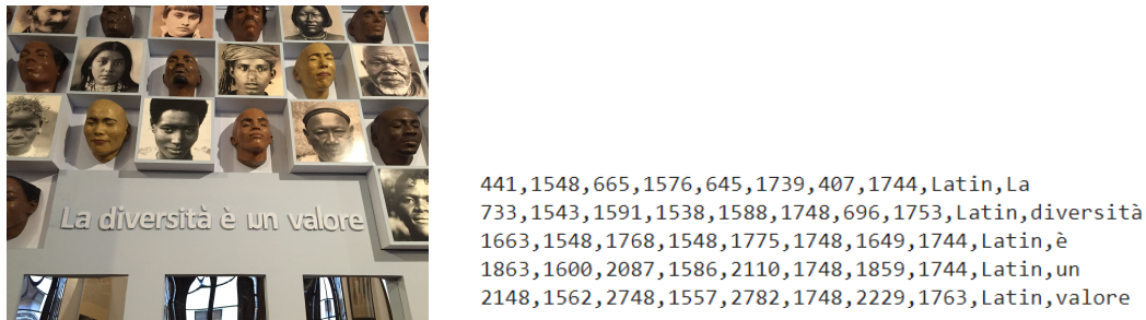
Figure 3.6: Example of ground truth information for an image from ICDAR2019. The structure of the file is the same for all the ICDAR datasets. For each word there is the prediction of the text and the corresponding location, annotated as a rectangle, which vertices coordinates are in clockwise order starting from the top. Note that in this dataset also the prediction of the language is present. The text that is not recognized is present in the ground truth file as ###.
