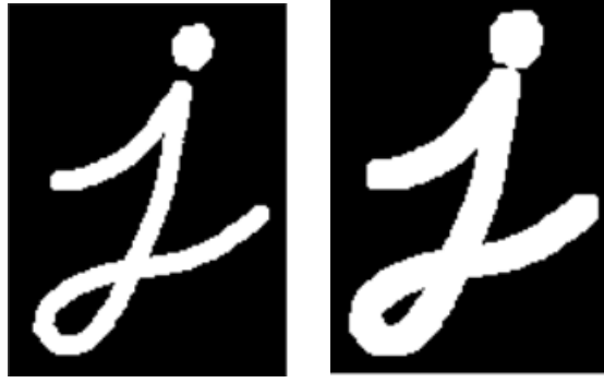
Figure 4.6: Left: original image (gray scale). Right: image after dilatation.
