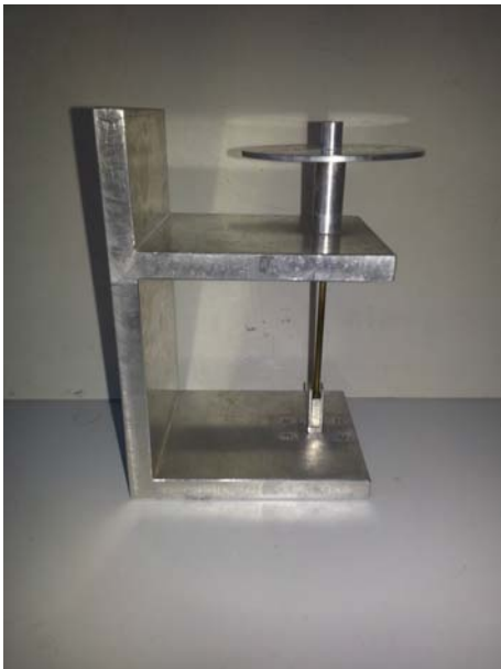
Figure 3.1: Plunger system that allows to calculate the cross section of the sample.
