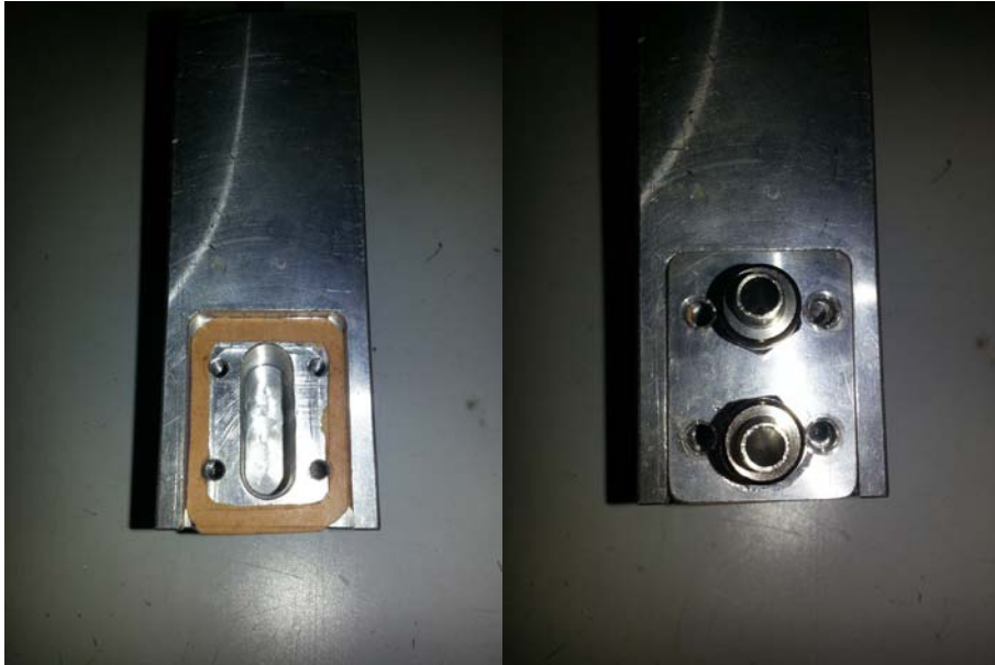
Figure 3.6: On the back of the main body is first cut and then is put a sheet of insulating material; in the right photo is subsequently added the lid. A hole is used to the liquid nitrogen entry and the other to vent.
