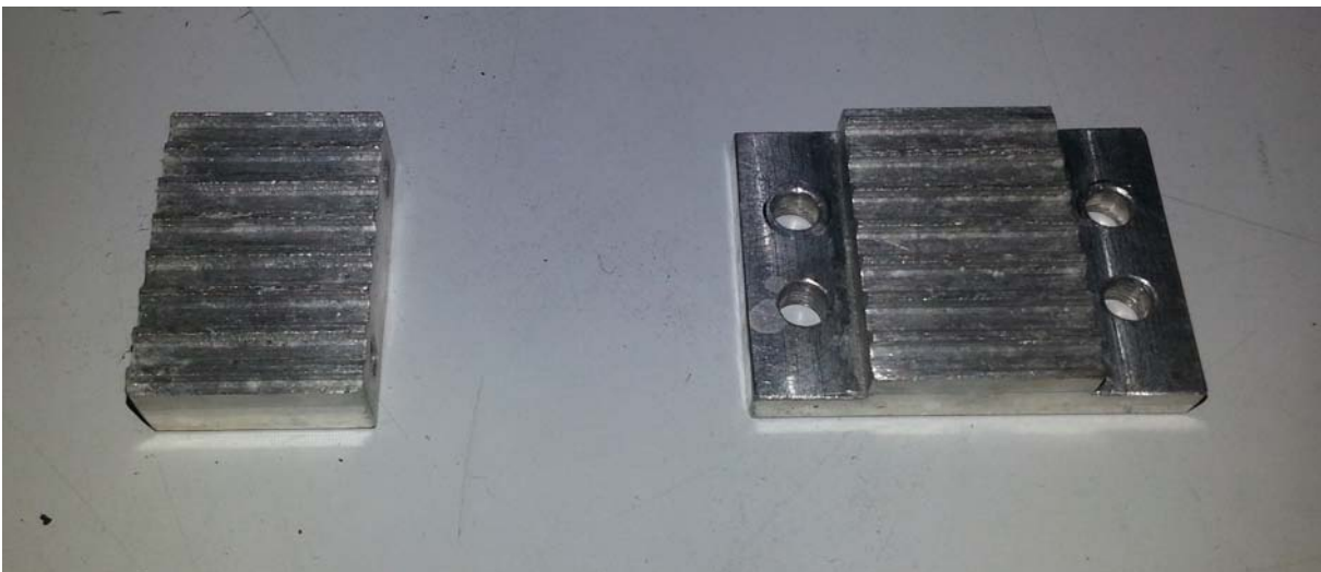
Figure 3.7: Notched plates; the left goes in front of the main body and the right one is removable.
