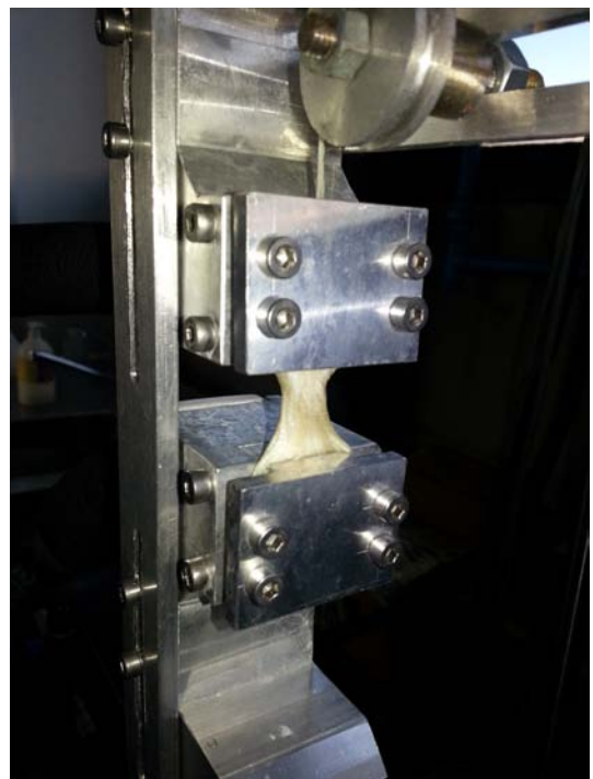
Figure 4.3: Placing procedure. First is close the bottom clamp and then the upper one.
