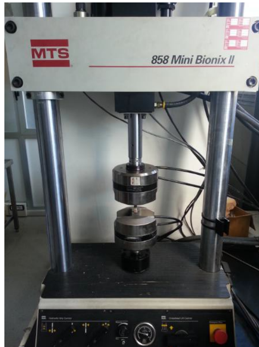
Figure 3.2: Specimen and puch gripped on the testing machine.
