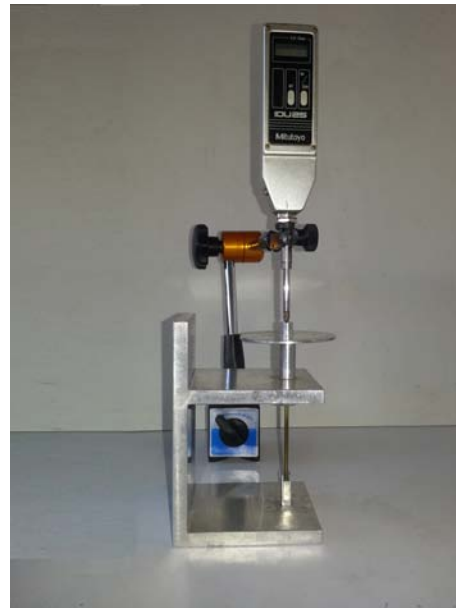
Figure 3.2: It can be noticed the positioning of the dial indicator, which must measure the displacement at the center of the plate.
