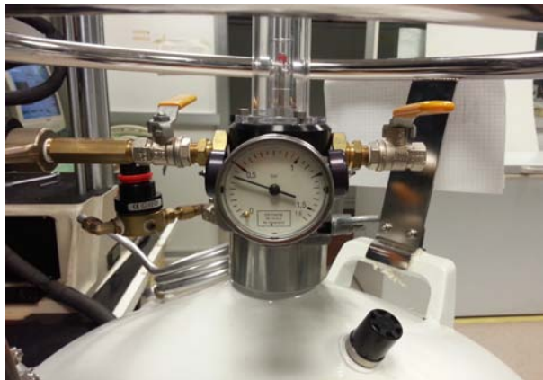
Figure 3.12: Particular of the valves and of the pressure (0,5 bar) gauge of the Dewar vase. The valve on the left allows the flow of liquid nitrogen, while the right (unused) allows the escape of vapours of nitrogen (warmer).
