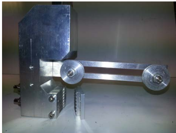
Figure 3.9: Upper assembled system. The removable plate is detached. The left pulley can move sideways to improve alignment.
