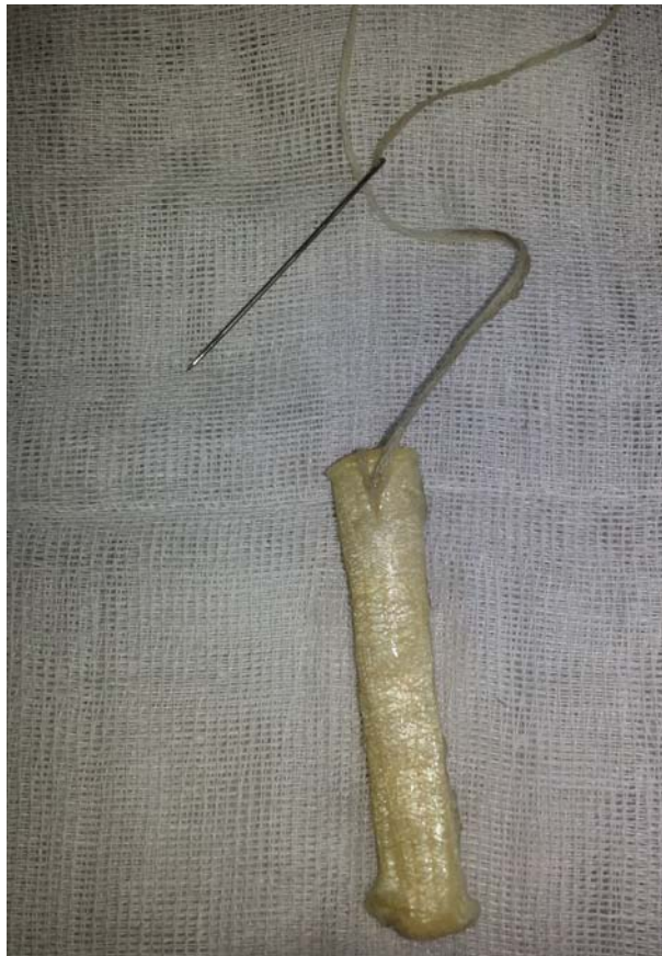
Figure 4.1: Sample sutured on a tip. The suture is useful for positioning on the clamps and eventually for pre-tensioning.
