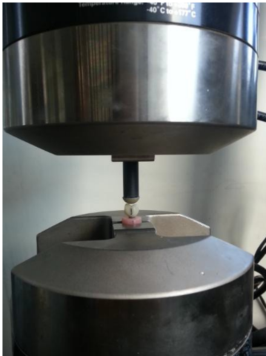
Figure 3.2: Specimen and puch gripped on the testing machine.
