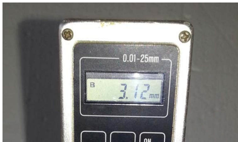
Figure 4.2: Section Measurement: The tendon is placed in the pit of the instrument and then is put on the plate light weight. On the dial indicator is shown the difference of height of the cursor (previously offset).
