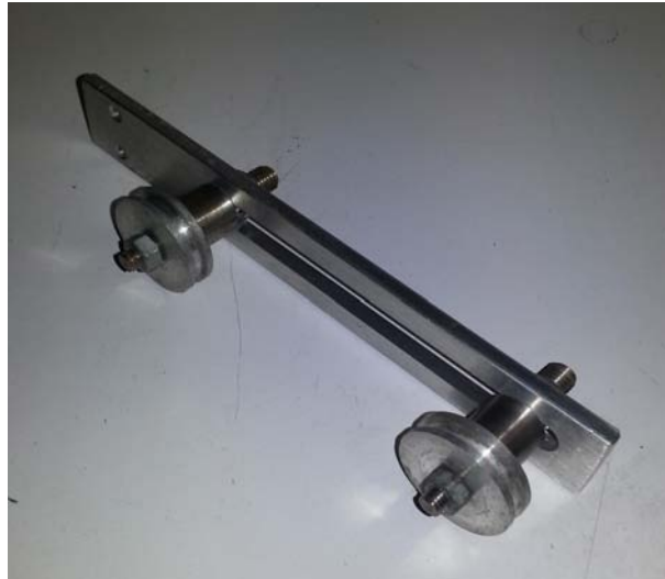
Figure 3.8: Pulley system; used to align the tendon and for the pre-tensioning.
