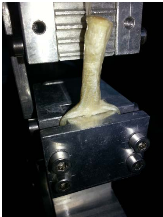
Figure 4.3: Placing procedure. First is close the bottom clamp and then the upper one.
