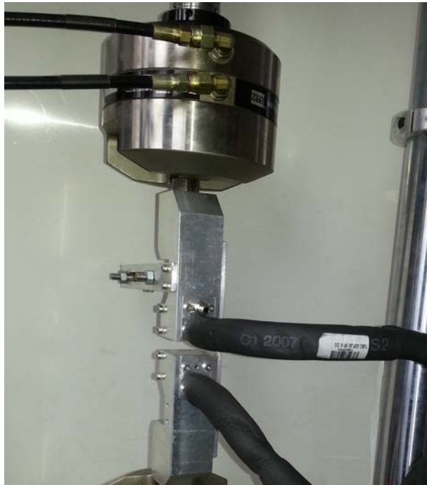
Figure 3.11: Detail of the rear of the clamp; the insulated pipelines in Teflon bring the liquid nitrogen in the refrigeration chambers in which the vaporization occurs. Locally, the temperature is maintained around -6^{\circ}\text{C} using the valve of the Dewar. Note the vent holes on the upper side of the lids.
