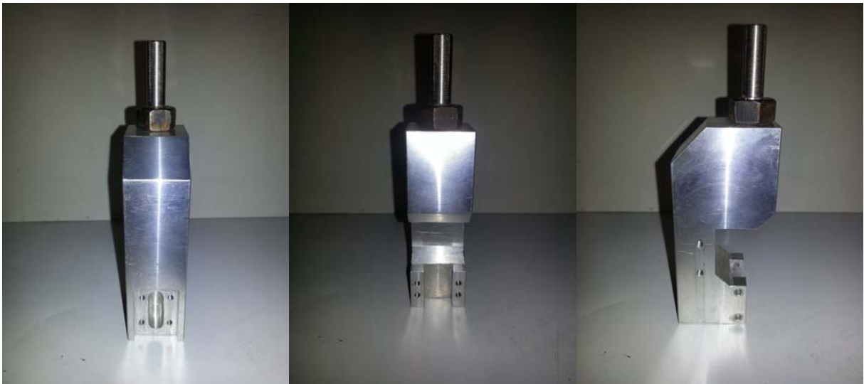
Figure 3.5: Rear, front and left views of the main body. Note, in the rear view, the chamber for nitrogen.
