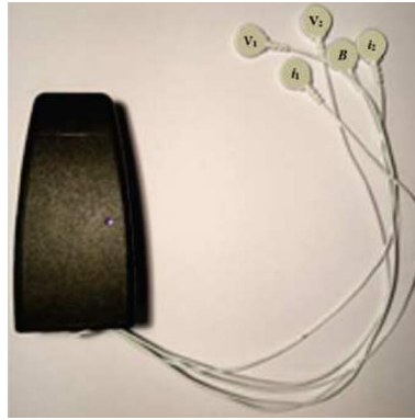
Figure 3.2: Holst Centre IBIS multifrequency bioimpedance monitoring unit
