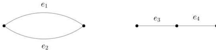
Figure 2.3: On the left we give an example of two edges  $e_1$  and  $e_2$  in parallel; on the right two edges  $e_3$  and  $e_4$  in series. Note that both the figures can represent a part of some given resistor network in which, as we said before, we are assuming that every edge has an associated quantity called resistance.
