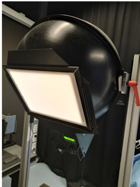
Figure 20: Light source used for the experiment (Esser Test-Charts Illuminator) in order to produce a smooth and diffuse light.
