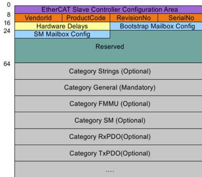
Figure A.4: Slave EPROM structure
