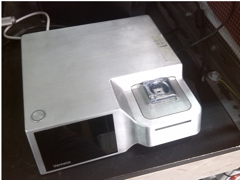
FIGURE 1.9: CAN-Q setup coupled with the chip support, put in the right slot.
