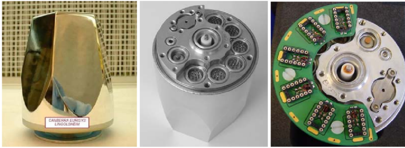
Figure 10: Pictures of the AGATA physically-unsegmented crystals. On the left the row germanium block, in the center the encapsulated crystal and on the right with the connectors PCB.
