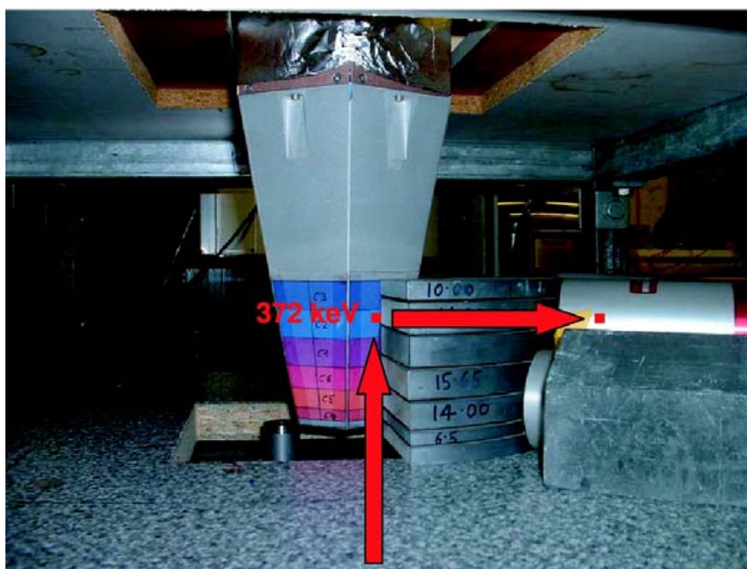
Figure 14: Photo of the scanning table in Liverpool. The lateral collimation and the BGO detectors are visible.
