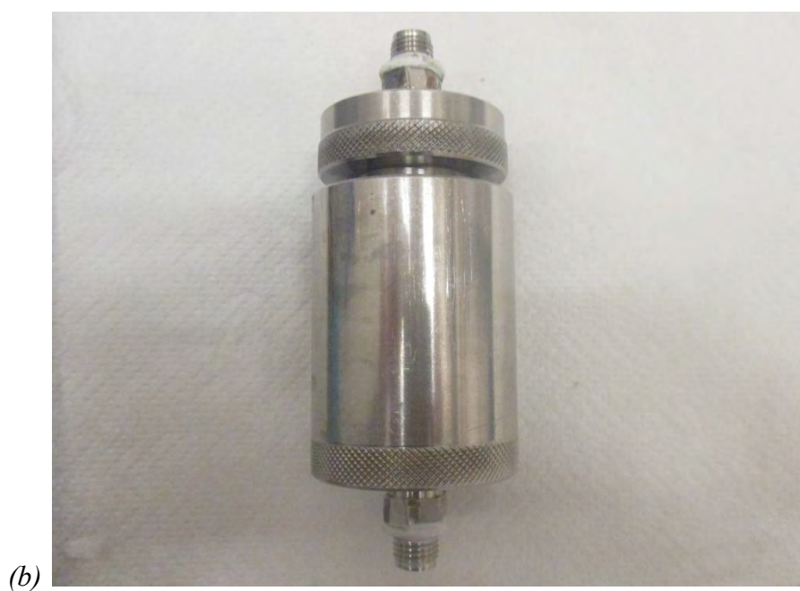
Figure D.1 (a) Two screwed parts of extractor (b) Extractor of the SFE used to extract phenols from asparagus
