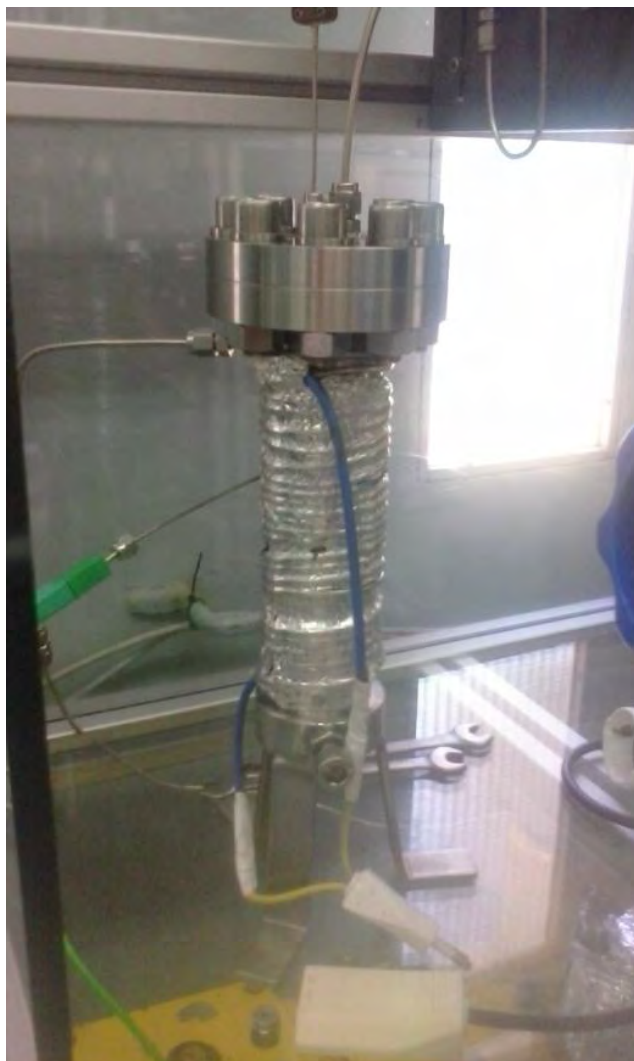
Figure B.1 Extractor of the plant used to perform the SFE of Malathion from chickpeas
