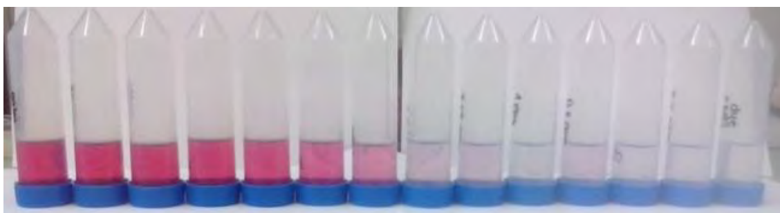
Figure.2.6. Comparison between the absorbance in different concentration of Malathion. From left to right: only dye-10-6-5-4-3-2-1.5-1.25-1-0.8-0.5-0.2-dye and NBS ppmv.
