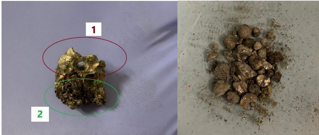
Figure 23 A clear distinction between the metallic phase and the residual slag : areas indicated by the number 1 shows the metallic phase while the residual slag is visible (left); metallic spheres separated from the sample (right).
