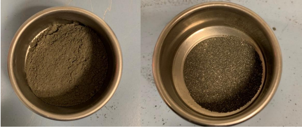
Figure 25 The pulverized slag after sieving for a smooth surface (tiny shiny particles of metallic phase is visible) (left); the slag (darker particles) + metallic phase (shiny particles) with the dimension of 180 \mu\text{m} (right).
