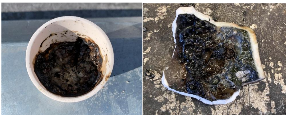
Figure 22 A close look at the crucible after cooling down (left); visible adhesion of the heated sample to the crucibles walls (right).
