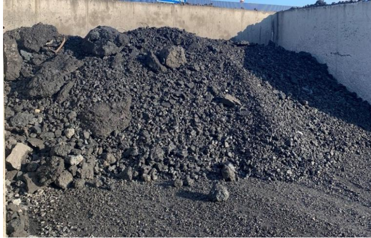
Figure 7 EAF slag generated in a steel plant.
