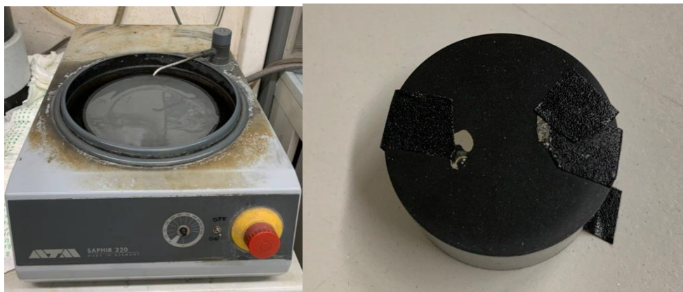
Figure 27 Polishing device, used to cut and shape the sample to desired size for an effective resin embedding (left), final sample embedded in resin (right).
