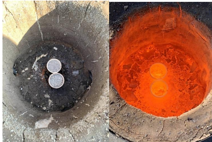
Figure 21 sample placement in the furnace (left), after the heating (right).
