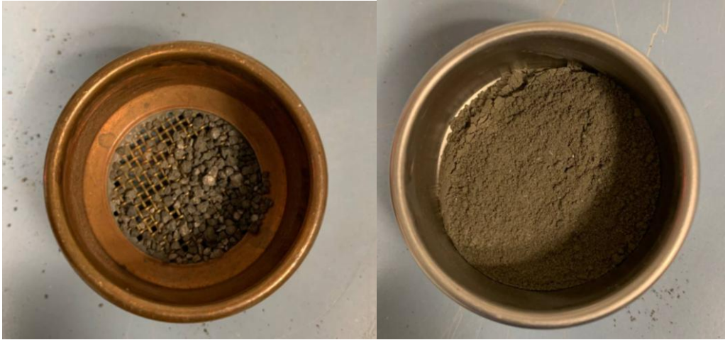
Figure 24 Continuous hammering, grinding and sieving enabled the bigger metallic material separation (left) from the residual slag (right).
