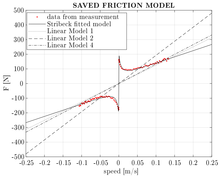
Figure 2.10: Comparison between experimental data, fitted Stribeck model and linear friction model. The latter is computed in three different ways.
