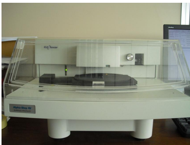
Fig. 5.4 – Profilometro KLA-Tencor Alpha-Step IQ
