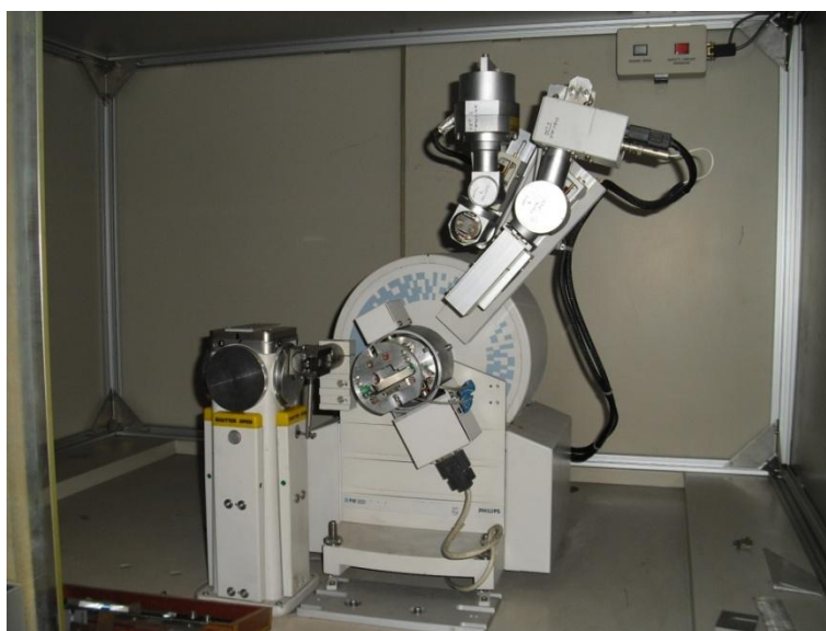
Fig. 5.18 - Diffrattometro Philips PW 3710
