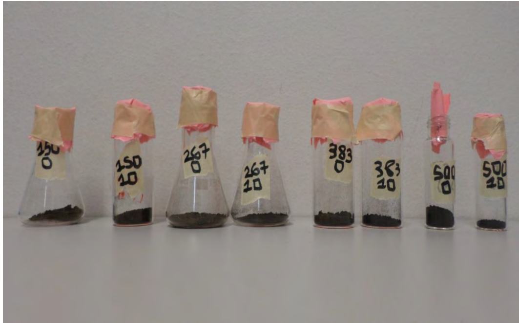
Figure 4.6. Photograph of the char after a pyrolysis at different temperatures and residence times.
