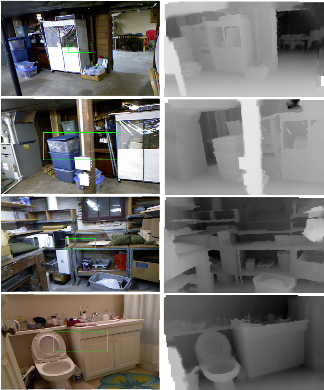
Figure 2.8: Processed sample from NYU Depth V2: The bounding box in green on the RGB images represent the collision box of the drone. Depth images have been colorized for visualization.
