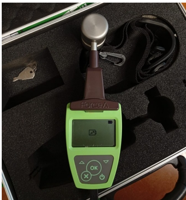
Figure 3.3: DUALEX SCIENTIFIC+™ instrument used for the non-destructive measurement of chlorophyll, anthocyanin, flavonoid indexes.
