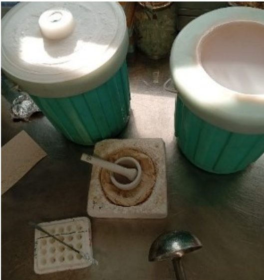
Figure 3.4: Equipment used for tissue grinding and sample preparation before RNA extraction, including mortars, pestles, spatulas and liquid nitrogen containers.
