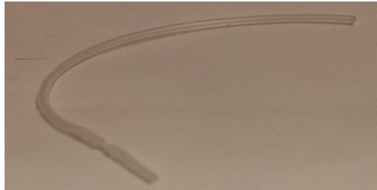
Figure 4.4. Connection between different ETFE and silicon tubes.
