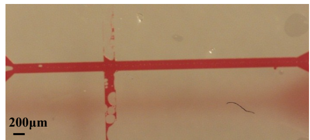
Figure 4.10. Water flow in the geometry with 45° cross-junction.
