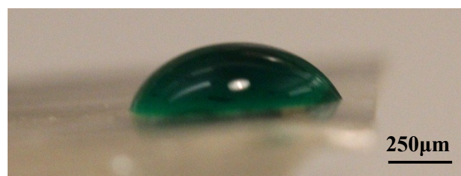
Figure 3.2. Droplet's profile upon unmodified OSTE(+) 80% material.
