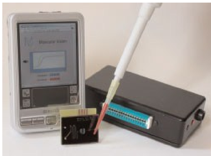
Figure 1.8. Molecular Vision's assay chip for polymer detection incorporating integrated organic photodiodes. Printed circuit board comprises amplifier and Bluetooth® connector for wireless data transfer to a PDA.
