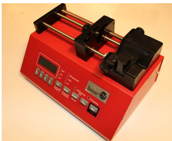
Figure 4.7. Programmable syringe pump(model 540060, from TSE systems, USA).
