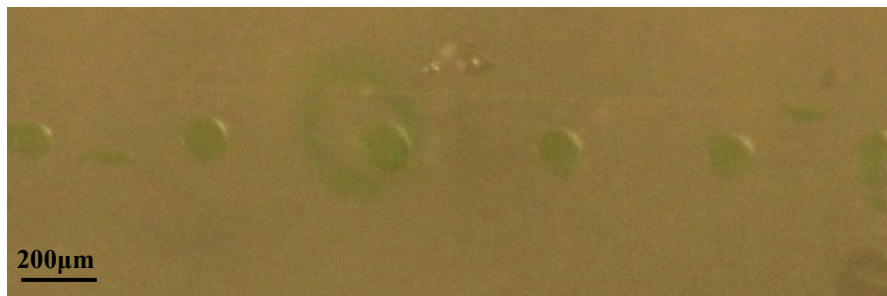
Figure 4.16. Train of droplets generated.
