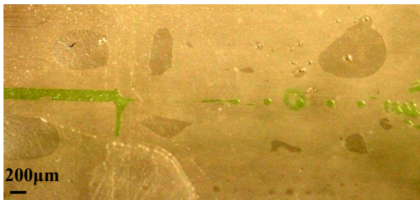
Figure 4.13. Breakup process in 90° cross-junction.
