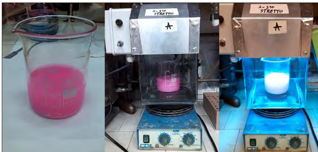
Figure 39: images of the equipment for photocatalytic degradation of Rhodamine-b in aqueous suspension
