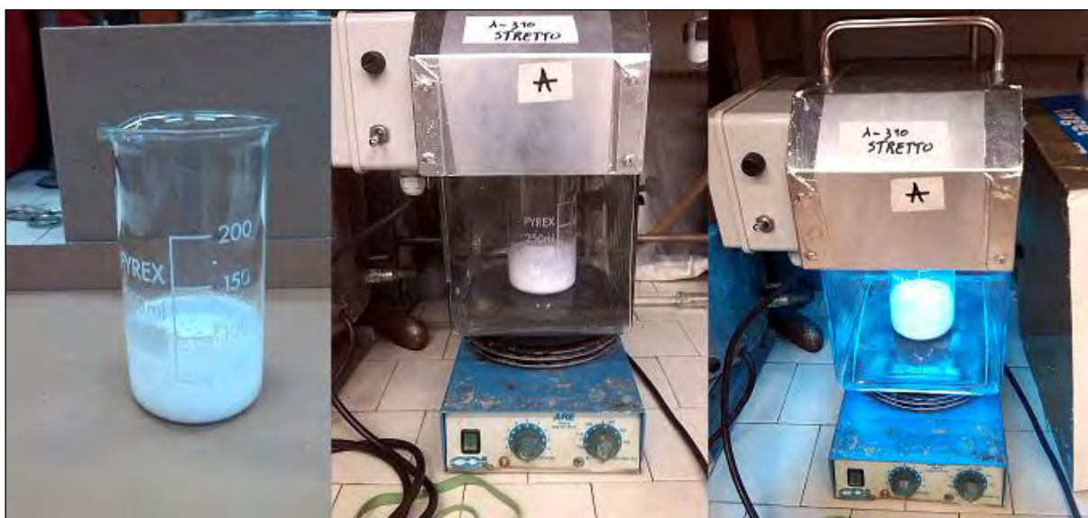
Figure 46: images of the equipment for photocatalytic degradation of a mixture of hydrocarbons in aqueous suspension
