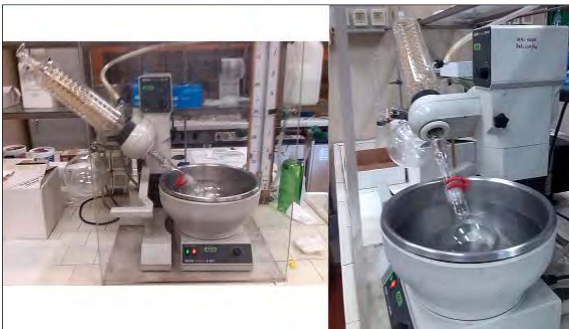
Figure 21: rotavapor BÜCHI Waterbath B-480
