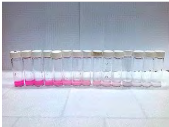
Figure 40: photodegradation of Rhodamine-b: gradual change of colour in function of the UV exposition time.
