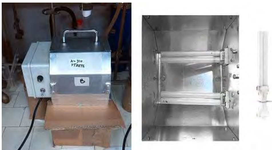
Figure 48: images of the equipment and UV lamps used for photocatalytic tests.
