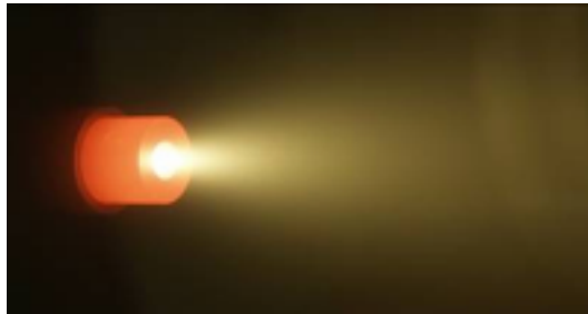
Figure 3.3: TALOS Arcjet operating with \text{NH}_3 , Universität Stuttgart [6].
