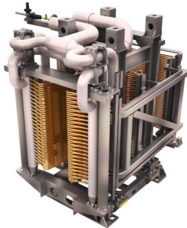
Figure 2-10 CAD view of MITICA's calorimeter
