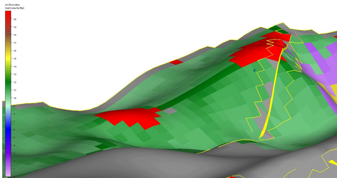
Fig. 8.2: Migri 3D view showing which structure are related with the two hydrocarbon accumulation visible in all the scenarios, I zone.
