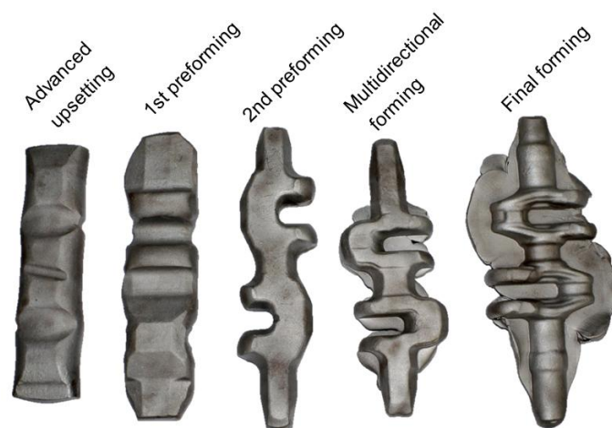
Figure 1.2 example of stages of forming process
