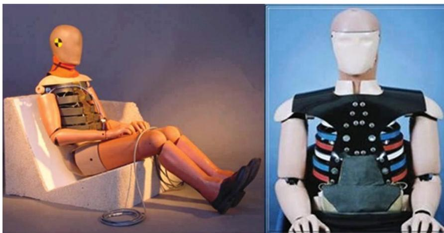
**Fig. 4:** Examples of dummies used in ATD simulations [6].
