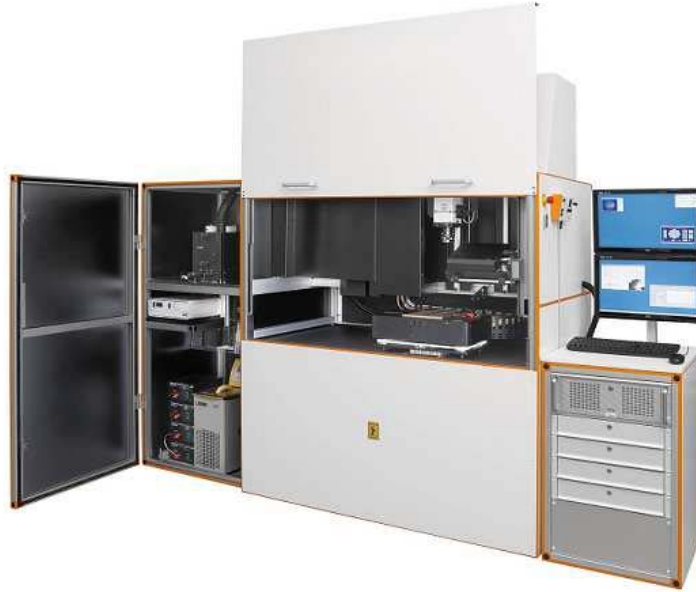
Figure 3.11: Instrumentation used to perform QE measurement.
