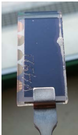
Figure 2.9: Good frontside. Enlightening the sample we can see that sample is almost uniform except the small border on the right.
