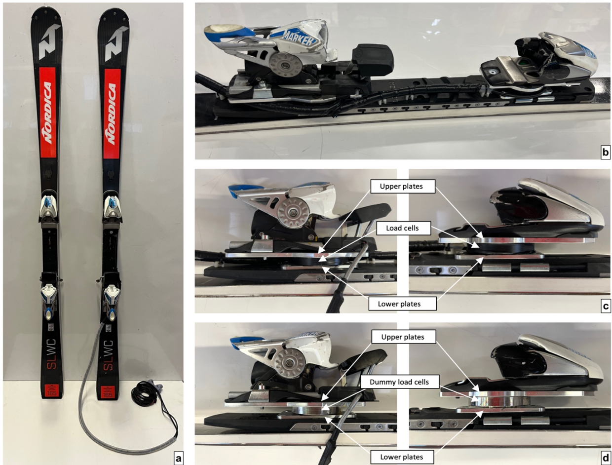
Figure 2.11. Instrumented slalom Nordica Dobermann SLWC 165 cm skis with Marker WC PC interface plate and Marker Comp 20.0 EPS bindings (a and b). Close up of the bindings on the instrumented ski (c) and the normal ski with the shims (d).
