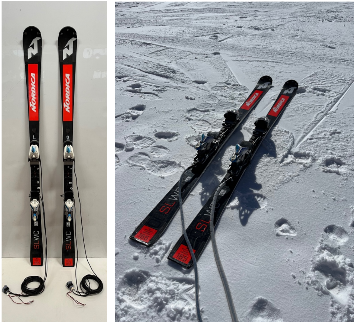
Figure 2.13. Instrumented Nordica Dobermann SLWC 165 cm skis
