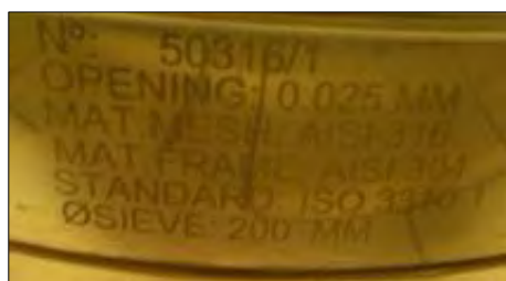
Image57: particular of the sieve Filtra N° 50316/1.
