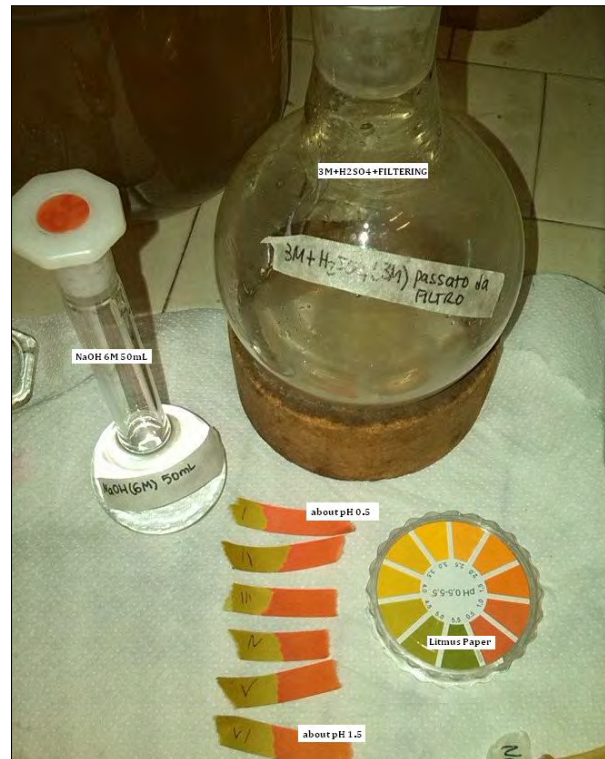
Image166: PH enhance with NaOH, paper test.
