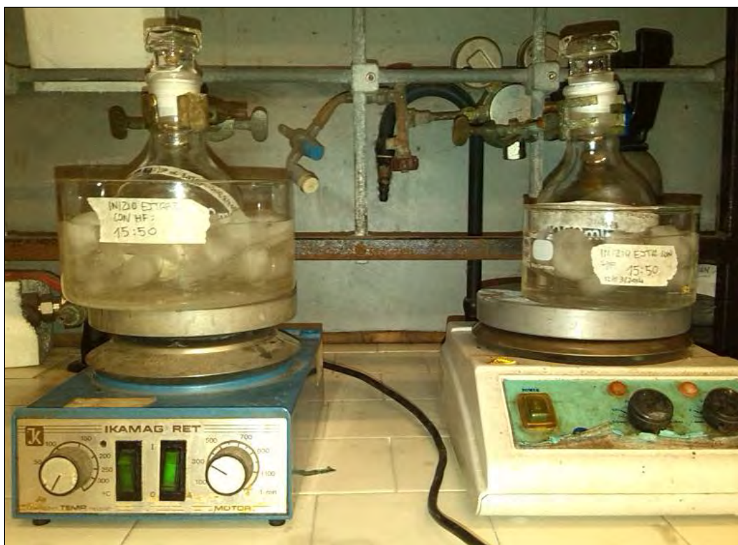
Image92: Two HF extraction with ice for the exothermic property of the reactions.
