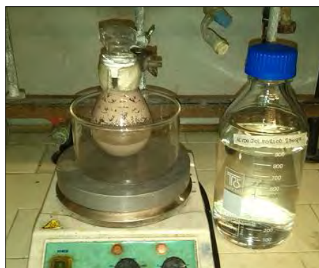
Image85: Start step of extraction.
