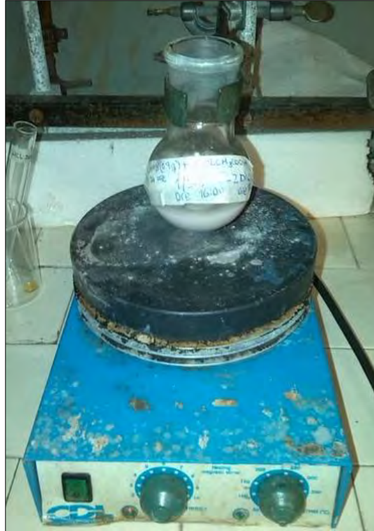
Image 143: Extraction from the solid HF3 with CH 3 COOH.
