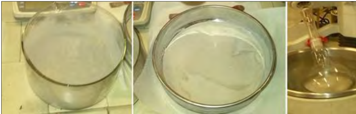
Image62: Result of the phase1, from left to right: fraction passed and settled, fraction held, liquid fraction.
