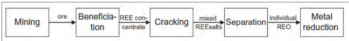
Image 15: Scheme of production Primary supply. Golev, A., Margaretha, S., Peter, E. D., Ali, S.H., Ballantyne, G. R., 2014. Rare earth supply chains: Current status, constrains and opportunities. Resources Policy 41 (2014) 52-59.
