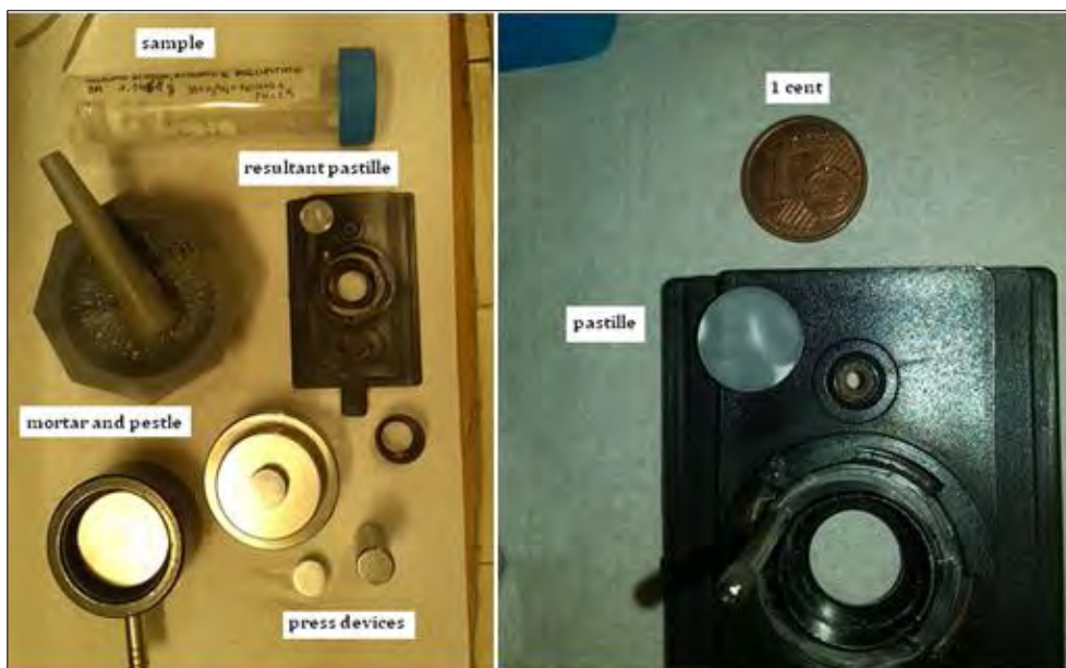
Image35: Instruments for the preparation of the pastille for the FT-IR analysis.
