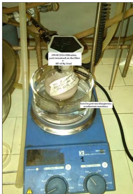
Image 123: Extraction procedure on LN1 with the addition of Hydrofluoric acid.
