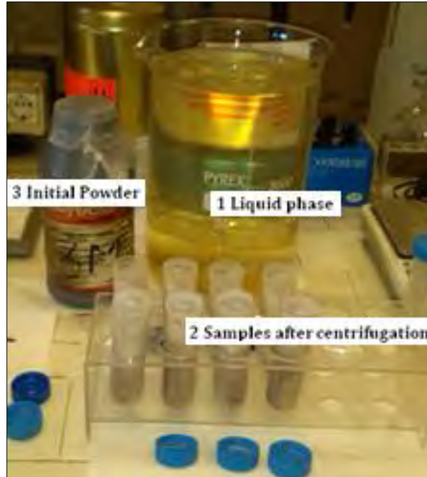
Image60:Detail of the fraction passes through the sieve (1 liquid phase after the centrifugation, 2 settled phases after the centrifugation, 3 starting material).
