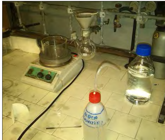
Image87: Filtration second step of extraction
