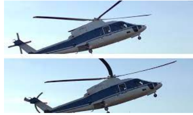
Figure 2.4: Differences between images acquired with a global and with a rolling shutter camera. Frame from a video of the official Sony youtube channel.
