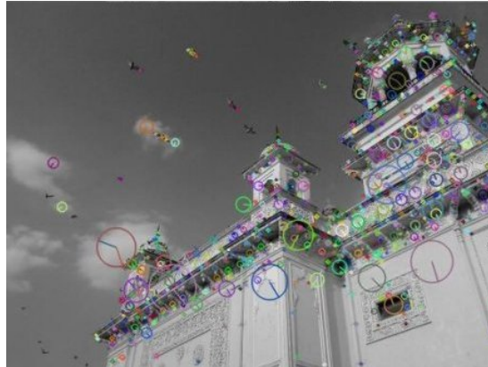
Figure 2.9: Image with SIFT features. In this representation the scale information is encoded in the dimension of the circles and the principal direction is described by the segment inside the circles. Image from the official OpenCV SIFT page [35].
