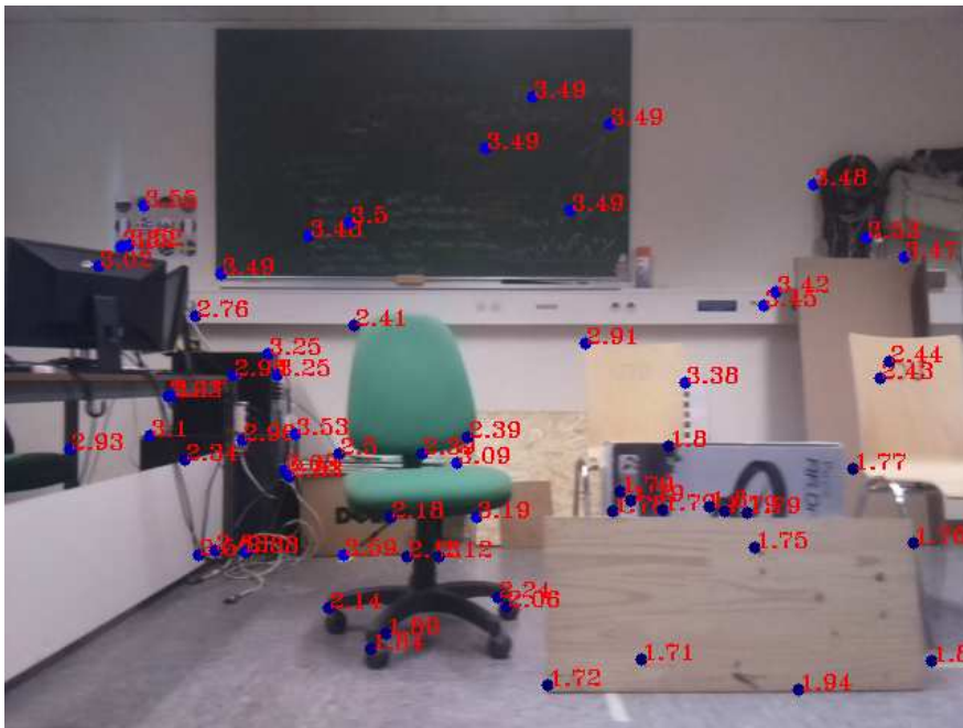
Figure 4.3: Example of an image with some of the detected orb features with the corresponding estimated distances. These images have been used to estimate the precision of ORB-SLAM3 with the actual experimental setup. The stability of the features between successive images allows us to check the synchronization of the RGB image with the depth map.
