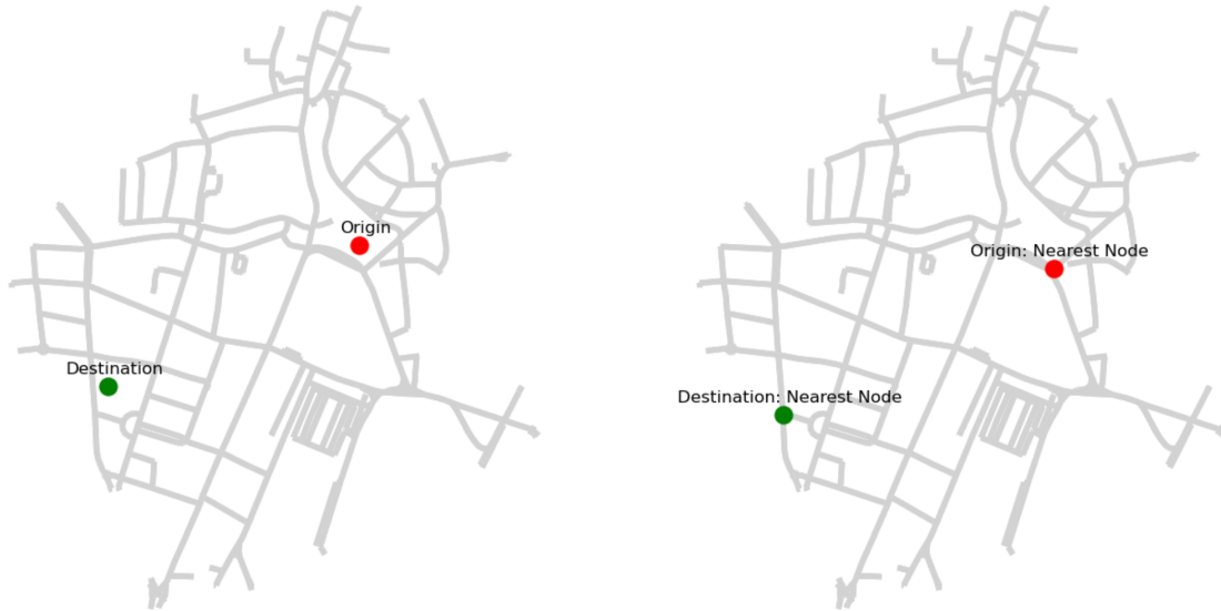
Figure 3.3: Nearest Node Calculation Step. The figure illustrates the process of mapping trip coordinates to the nearest nodes in the network.
