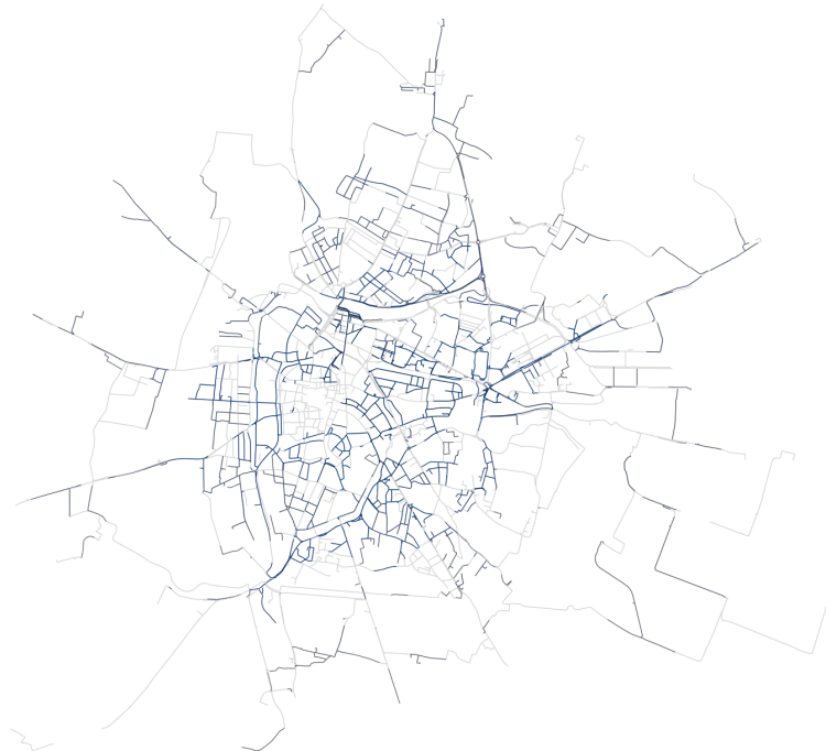
Figure 4.4: Components Identification. Legend: Light gray lines represent routes with bike paths. Blue lines represent component edges.
