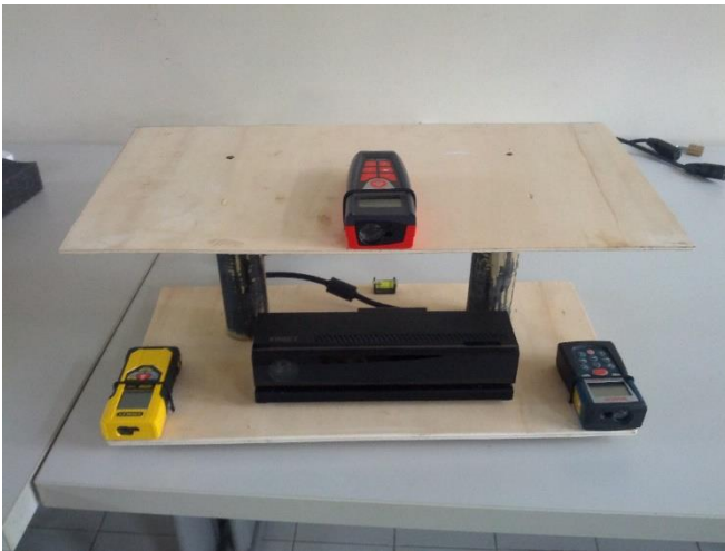
Figure 39 - Platform with three laser meters and a Kinect One
