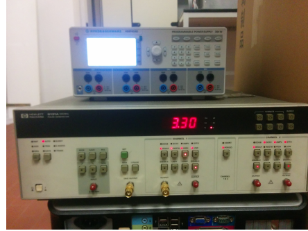
FIGURE 5.6: Power supplies: on top power board/GCU power supply; on bottom the pulser used for the LED light. Only one channel has been used.
