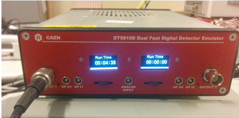
FIGURE 5.1: CAEN DT5810D Dual Fast Digital Detector Emulator.
