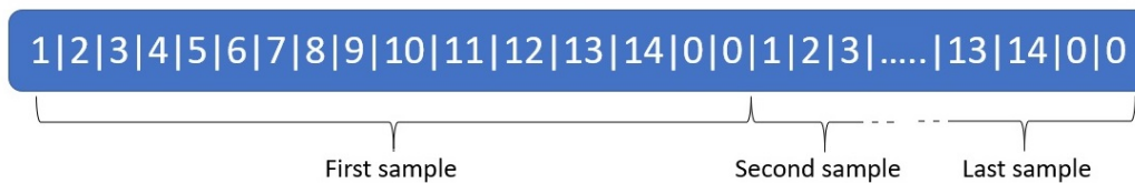
FIGURE 4.14: Scheme of the bit adjustment by the ordering module.
