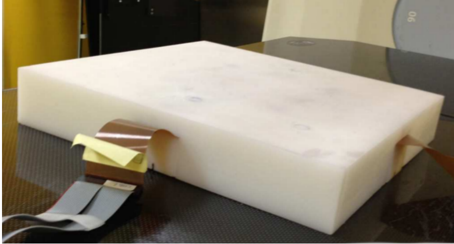
Figure 3.2: The slab phantom containing the DSSSSD, placed on the treatment couch at the Virgen Macarena Hospital.
