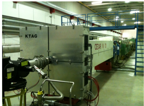
Figure 3.2: The CEDAR-W installed on the NA62 beamline with new 64 PMT light collection system
