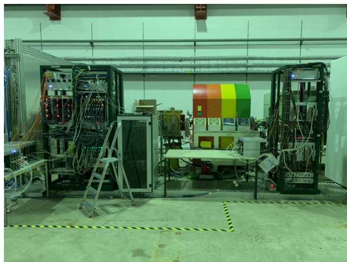
Figure 7.17: General view of the Veto Counter station in the experimental hall. The rainbow module in the middle is the TCX collimator, stations are located at either side of it while the racks contain all the required power supplies and readout modules.
