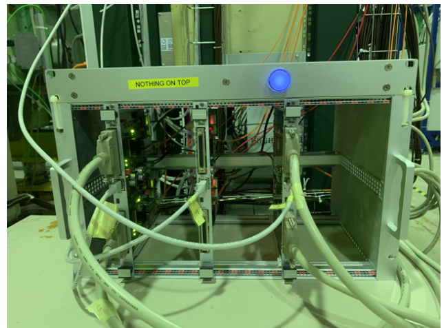
Figure 7.16: The TDC modules for FELIX readout
