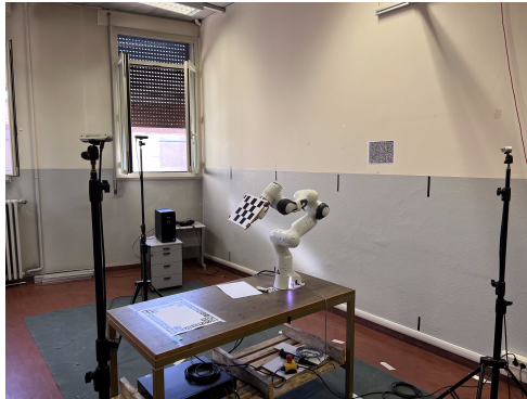
(a) Robotic workcell equipped by a camera network of depth sensors D455, arranged around the robot arm placed on the center of the workcell.
