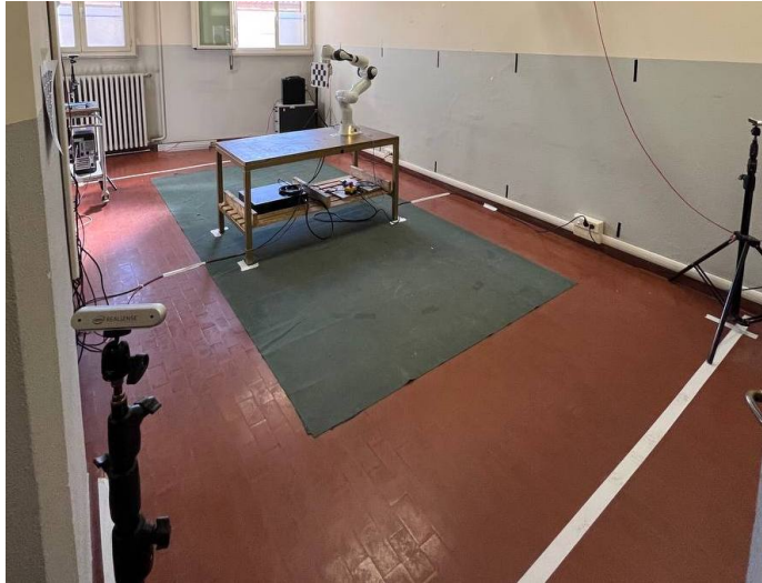
Figure 6.12: Robotic workcell designed in Robot Vision Lab; in particular in this image there are three depth sensors D455 with a robot arm in the center of the workcell with the chessboard attached on the end-effector.
