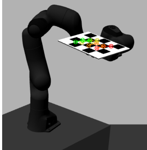
(b) Wrong checkerboard detection due to the high checkerboard tilt.
