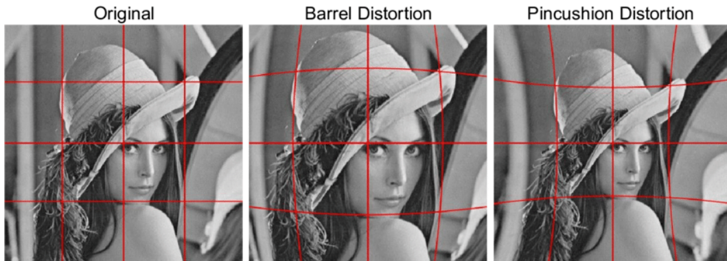
Figure 3.12: Comparison among the original image at the left, its barrel distortion and at the right the pincushion distortion.
