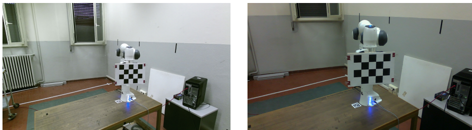
(a) Checkerboard image captured by the Kinect V2 at a distance d = 1.2 m.
