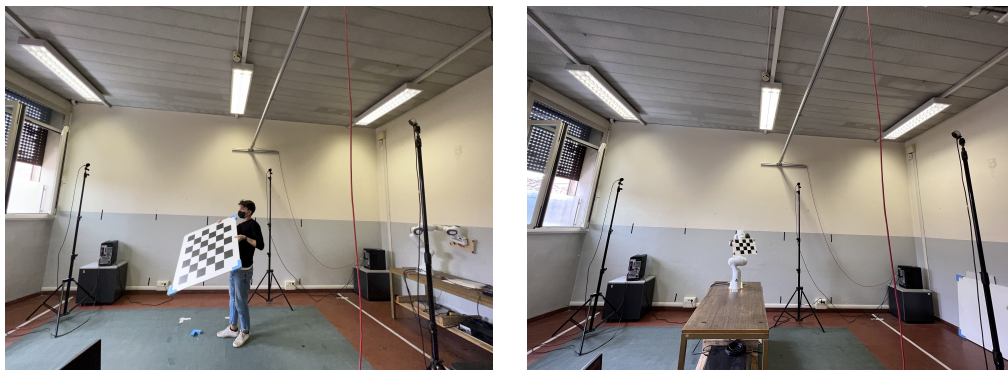
(a) Manual images acquisition phase for OpenPTrack calibration. (b) Automatic images acquisition phase for our proposed calibration method.
