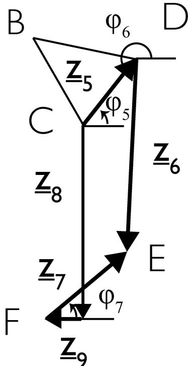
$$\underline{z}_5 + \underline{z}_6 - \underline{z}_7 - \underline{z}_8 - \underline{z}_9 = 0$$
