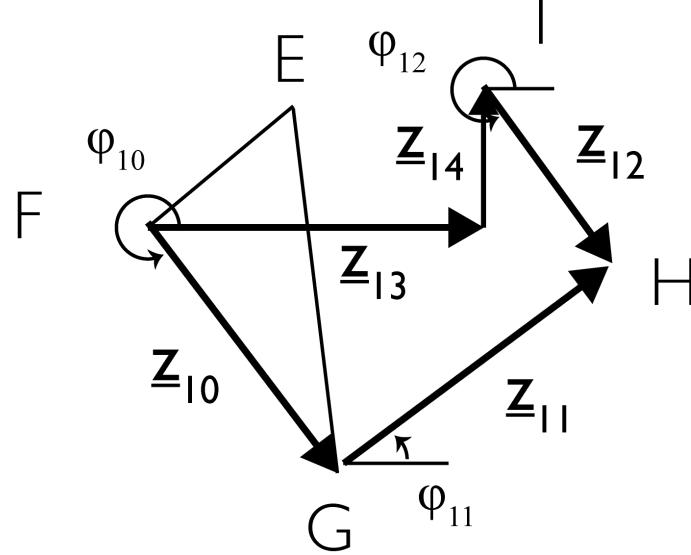
$$\underline{z_{10}} + \underline{z_{11}} - \underline{z_{12}} - \underline{z_{14}} - \underline{z_{13}} = 0$$
