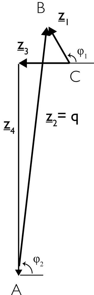
$$\underline{z}_2 - \underline{z}_1 + \underline{z}_3 + \underline{z}_4 = \underline{0}$$
