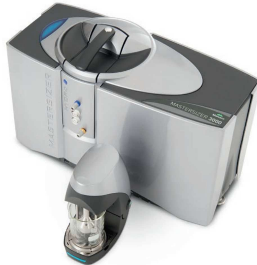
Figure 5.5: Mastersizer Hydro EV device.
