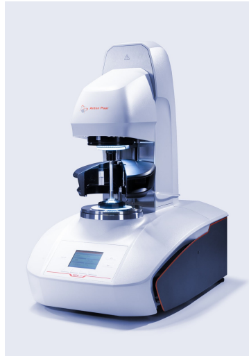
Figure 5.13: Anton Paar MC92 rheometer.
