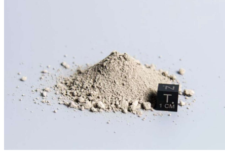
Figure 2.10: LMS-1D Simulant, photo credit Matthew Villegas[72].
