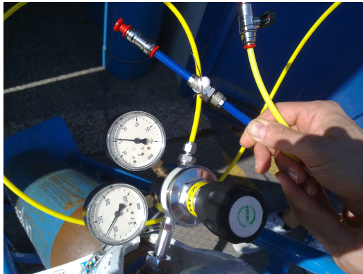
Fig. 4.6: Testing the prototype with helium up to 20 bar.
