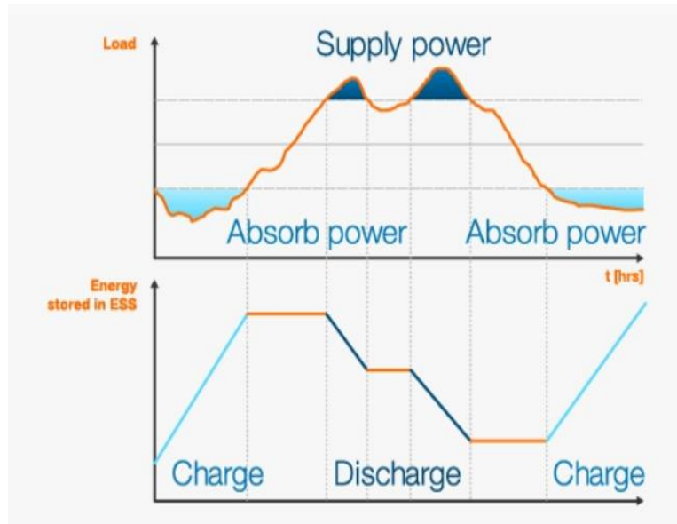
Figure 1-5 Discharging EES for Load Leveling
