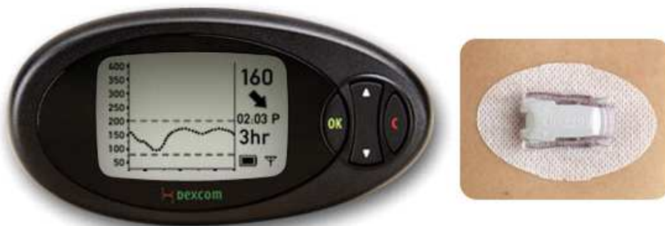
Figure 1.4: DexCom SEVEN . Left: the receiver. Right: subcutaneous sensor and transmitter[15].
