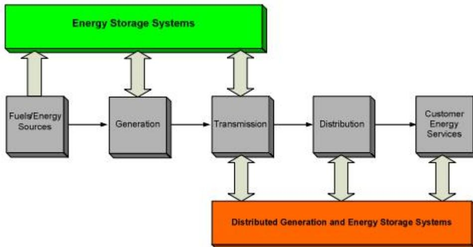
Figure 1.6: Electricity value chain with energy storage as the sixth dimension, source: Energy Storage Council (ESC)
