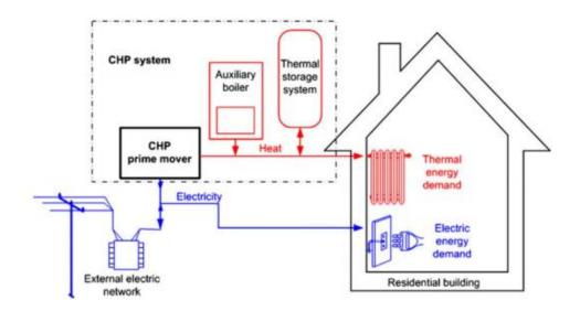
Figure 1.4: Typical integration of mcro-CHP system in a residential building, by Martines et al., 2017
