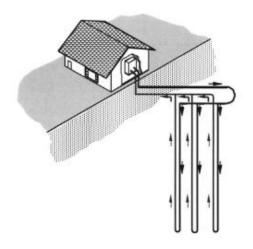
Figure 1.5: Vertical ground-coupled heat pump, by Phetteplace, 2007 *Fuel cells*
