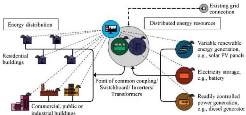
Figure 1.7: Structure of micro-grid, by Ting et.al., 2021
