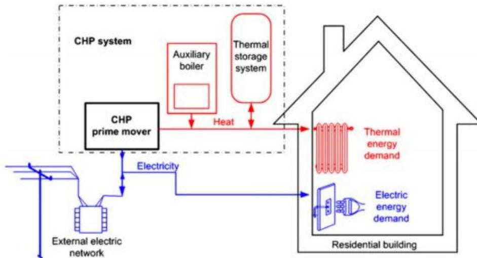
Figure 1.4: Typical integration of micro-CHP system in a residential building, by Martines et al., 2017
