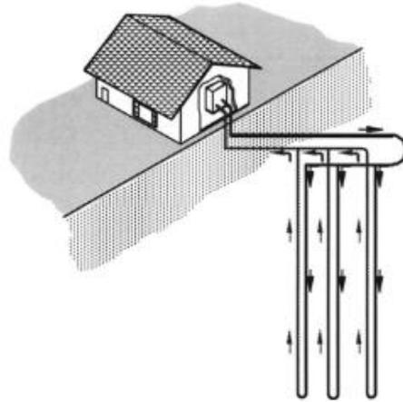
Figure 1.5: Vertical ground-coupled heat pump, by Phetteplace, 2007
