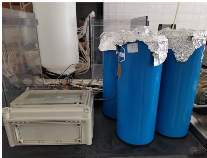
Figure 3.15: Dewar vessels ready for the self-heating test
