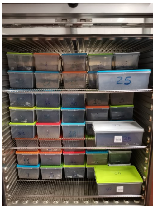
Figure 3.25: reactors stored at 58°C in the oven
