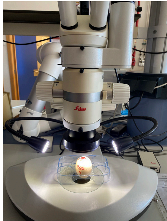
Figure 3.15: Leica MZ APO X16 magnification microscope utilized for the verification of angiogenesis in the embryos.
