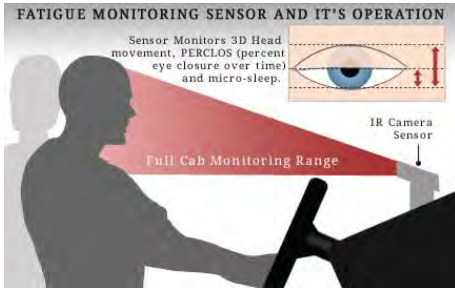
Figure 2: PERCLOS technology working scheme. Source: [24]
