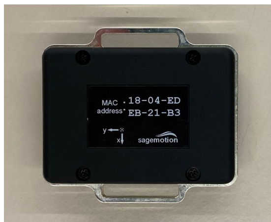
Figure 3.2: Reference system and identification code of a SageMotion node
