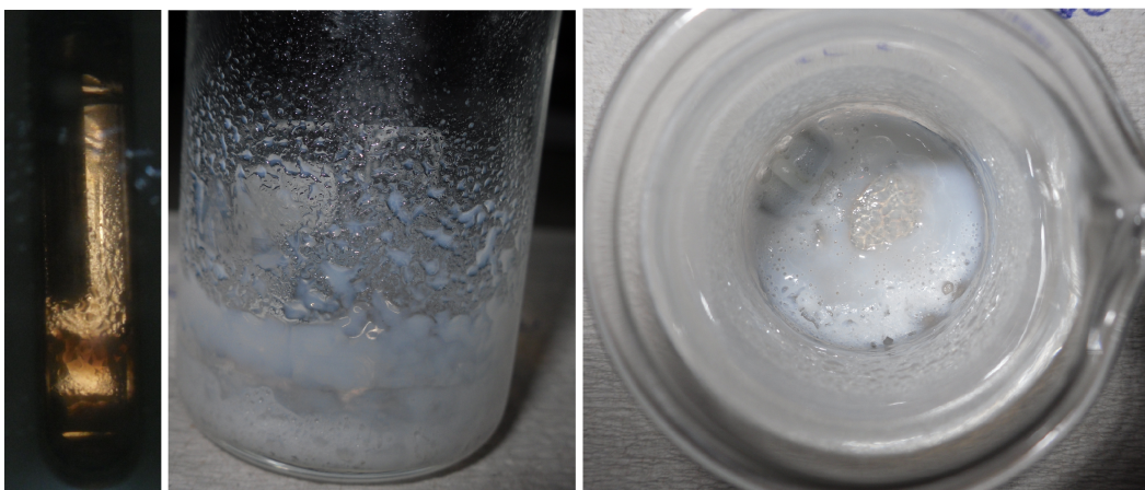
Figure 3.5: Ibuprofen sodium salt melted, after pressurization with carbon dioxide at 41°C and 70 bar. The drug is still liquid, at ambient condition. First picture on the left: melt drug inside the view cell, under pressure. Picture in the middle: melt drug in the beaker, seen from the side. On the right: same beaker seen from above.
