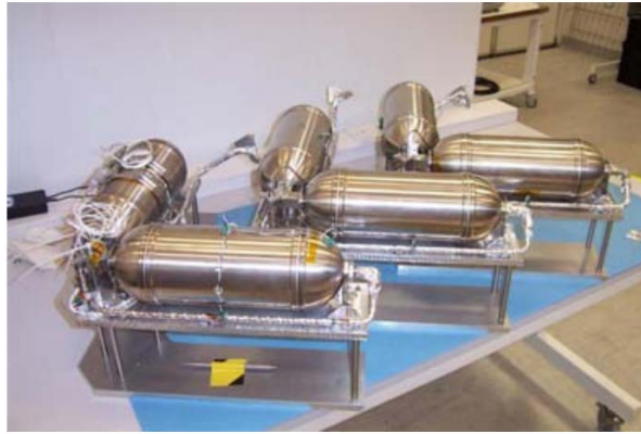
Figure 2.2: DMC butane propulsion system [19]
