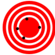
Figure 5.1: High accuracy but low precision.
