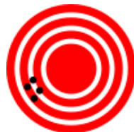
Figure 5.2: High precision but low accuracy.
