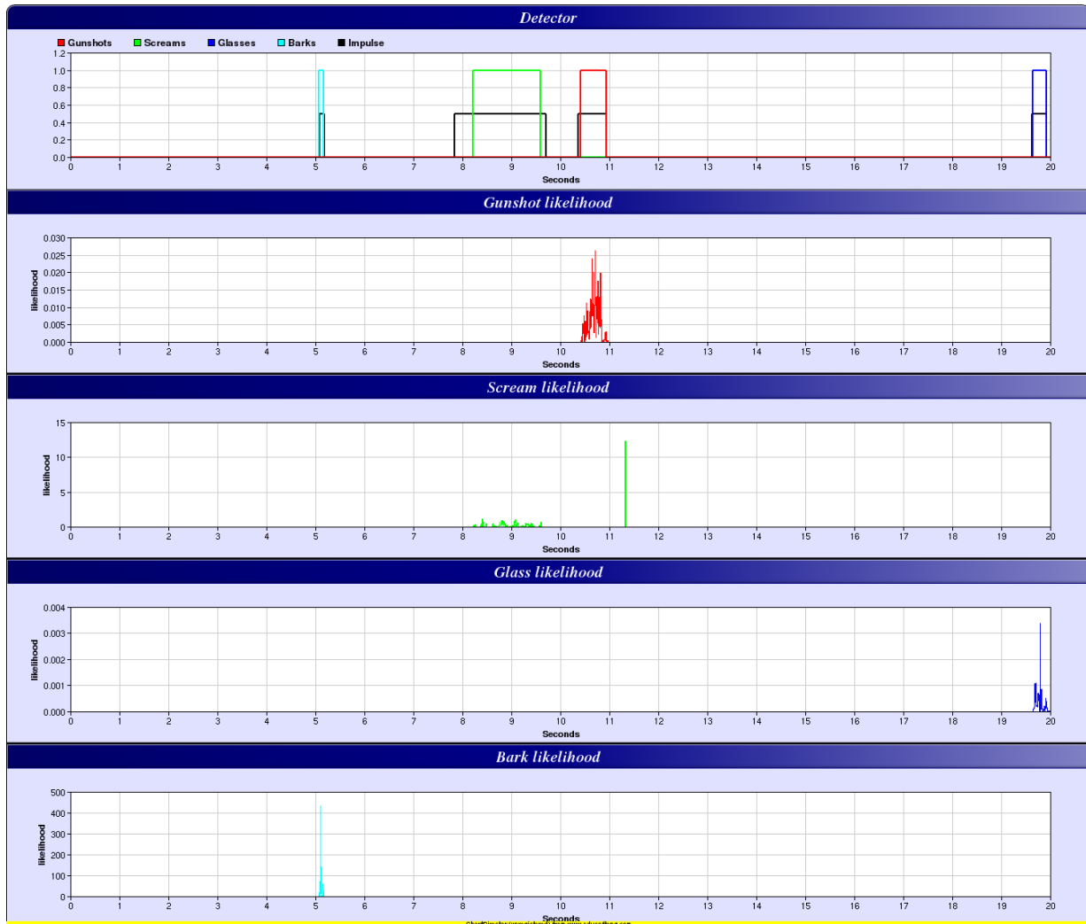
Figure 3.1: Visualization of likelihood and detection in time. The upper plot is the detection over the time and in the other plots there are the values of the likelihood of each model. Legend: black - impulsive sound; red - gunshots; green - screams; blue - broken glasses; light blue - barking dogs.
